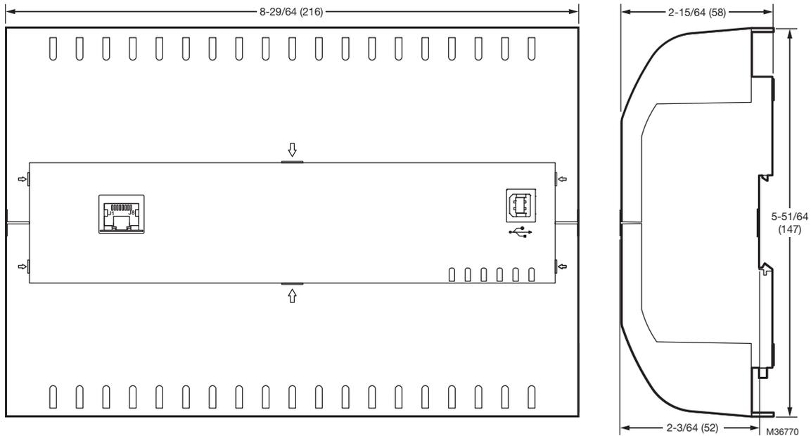
**Fig. 8. EagleAX Controller with covers, dimensions (in mm).**
