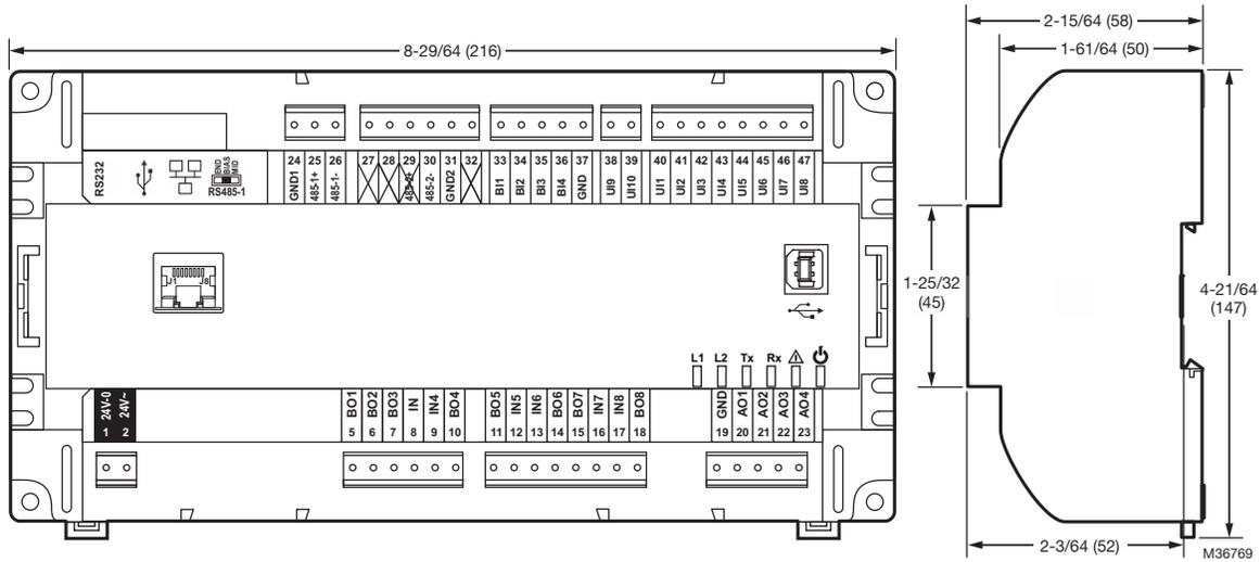
**Fig. 7. EagleAX Controller (shown: model with onboard I/Os), dimensions (in mm).**
