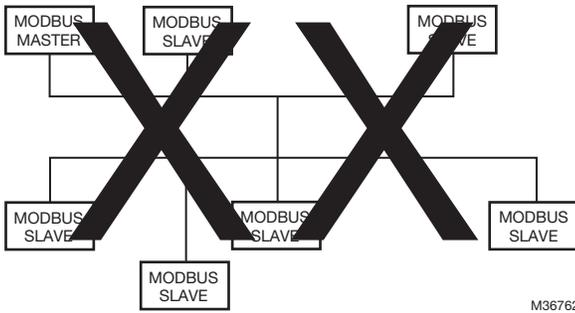
**Fig. 6. Prohibited Modbus wiring topology (example).**
